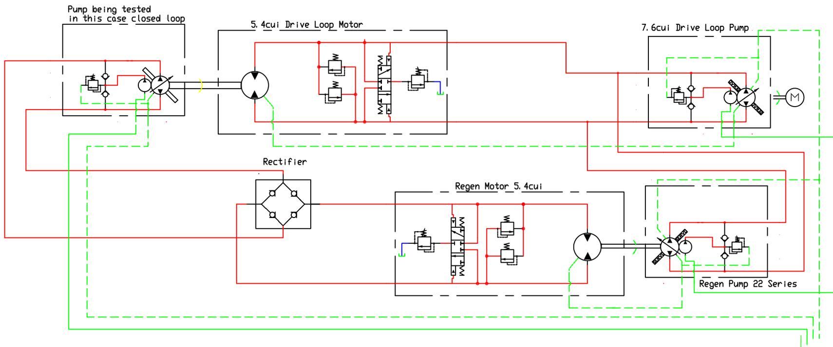
6way selector for pump/motor test in drive loop not shown, loop filters, flow meters, gauges left out for clarity. Aux pump for charge when required not shown.
